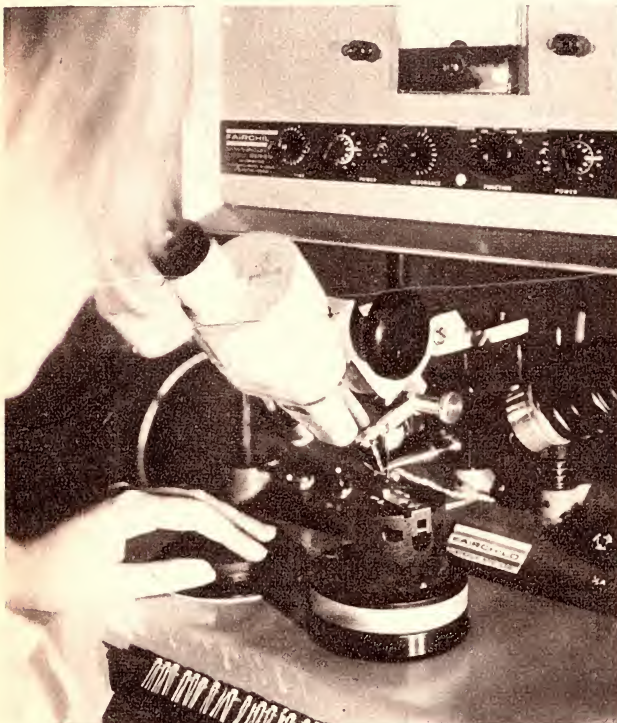
With the aid of a binocular microscope, an operator attaches the tiny wires which connect the emitter and base of the dice to the external connecting leads. These are part of the "header" assembly, to which the dice is attached.
